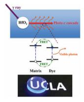
An efficient multigram-scale single-precursor synthesis of high-quality hafnium oxide nanoparticles is reported. After surface modification, these nanoparticles are used to fabricate highly transparent nanocomposite monoliths (2 mm thick,  $T_{\rm 550~nm} > 75\%$ ) at loadings up to 40 wt%. The nanocomposite monoliths are efficient in detecting gamma radiation, being capable of producing a full energy photopeak with deconvoluted resolution <8%.
