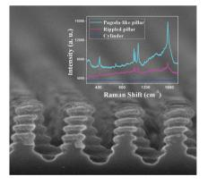
Arrays of pagoda-like nanopillars are created by employing a standing wave during phase-shift interference lithography. A series of metallic nanogaps on the side walls of the nanopillars provide a high density of hot spots for the localization of the electric field, thereby making the arrays an effective surface-enhanced Raman scattering substrate. The arrays can be further micropattened by photolithography, enabling the analysis of multiple samples on a single substrate.
