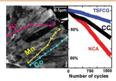
Two-sloped full concentration gradients (TSFCG) of Ni, Co, and Mn ions throughout the cathode particles to maximize the average Ni concentration are successfully synthesized via coprecipitation. The TSFCG cathode exhibits the best cycling stability compared to conventional cathode and  $\text{Li}[\text{Ni}_{0.8}\text{Co}_{0.15}\text{Al}_{0.05}]\text{O}_2$ , which delivers a discharge capacity in excess of 200 mAh g<sup>-1</sup> with excellent cycle life and thermal stability.
