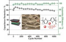
By a doping polypyrrole film supported on functionalized partial-exfoliated graphite (FEG) substrate with  $\beta$ -naphthalene sulfonate anions, the polypyrrole electrode achieves a remarkable capacitance retention rate of 97.5% after cycling between -0.8 and 0 V versus saturated calomel electrode for 10 000 cycles. An asymmetric pseudocapacitor using the stabilized PPy film as anode can also retain 97% of capacitance after 10 000 cycles.
